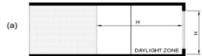
(a) Section view (b) Plan view of daylight zone under a rooftop monitor
